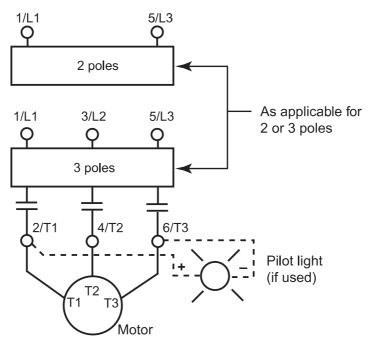
**NOTE:** The lamp is polarity sensitive in DC applications.
