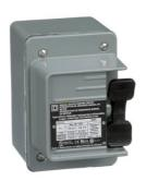
Switch, manual, 30A, 3 pole, 20HP at 575VAC, 3 phase, toggle operated, no indicator, NEMA 4, one conduit opening
